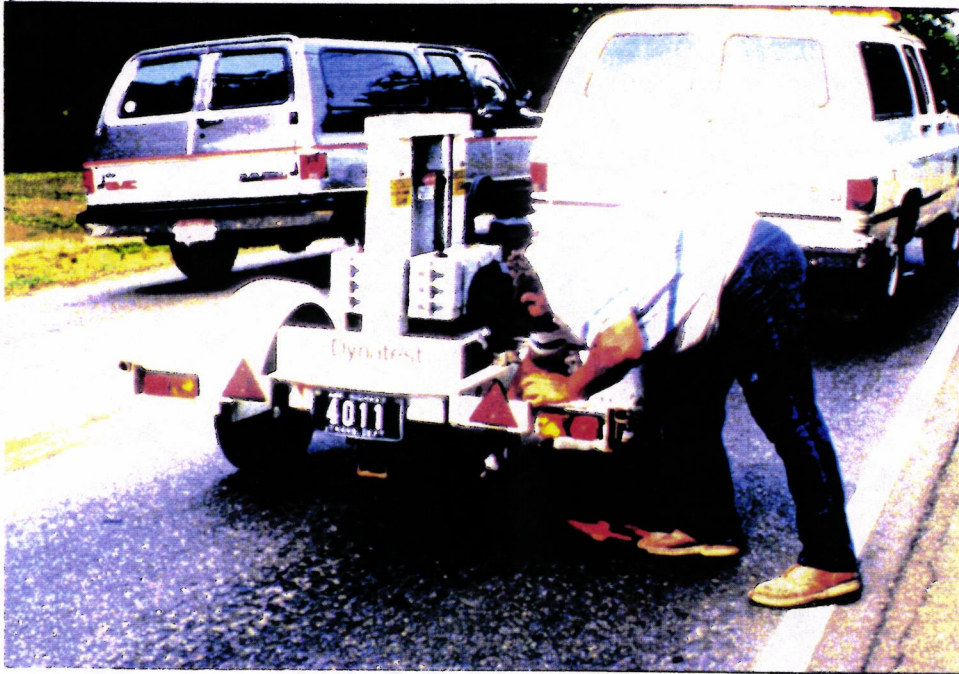
Falling Weight Deflectometer at Magnolia
